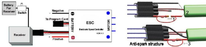
**Note**: There are 2 control wires on the HV controller. The longer one is close to the positive battery wire, which is connected with the receiver, and the shorter one is close to the negative battery wire, which is used to connect the program card to set the programmable parameters of the controller.
